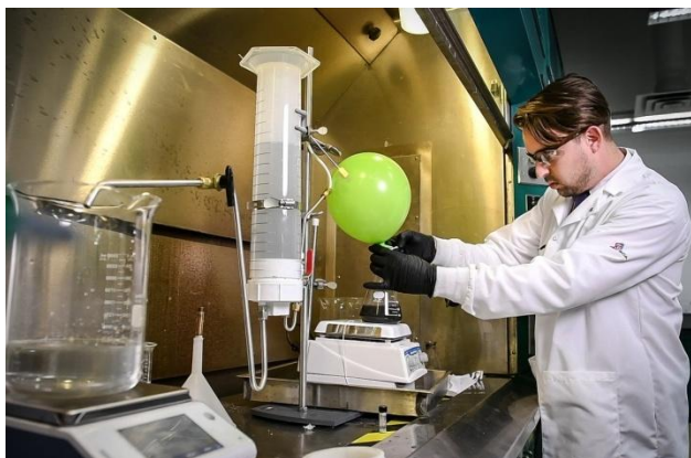
In a demonstration, Army researcher Anthony J. Roberts powers a radio-controlled toy tank with hydrogen harvested from a unique chemical reaction. Scientists and engineers have found a way to split hydrogen and oxygen quickly and without a catalyst, resulting in high amounts of energy.
